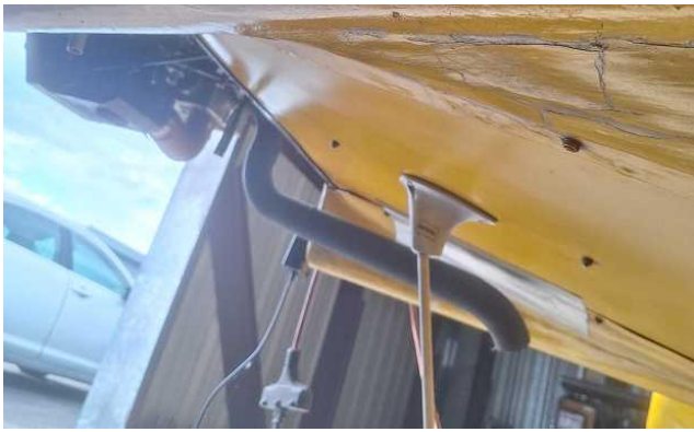
Fig. 15: Lucky fit of the exhaust pipe under the Jodel fuselage. I'd rather be lucky than good! Note the small heat shield just above the exhaust pipe.
