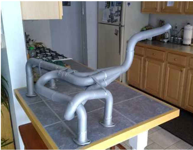
Fig. 11: Exhaust system after sandblasting. The bracing between individual runners is more visible in this shot.
