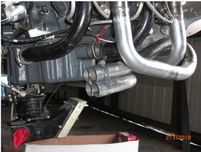
Fig. 7: The number 3 runner has been final welded. All four runners are now fitted, final welded and in good position for welding into the 4-into-1 collector.
