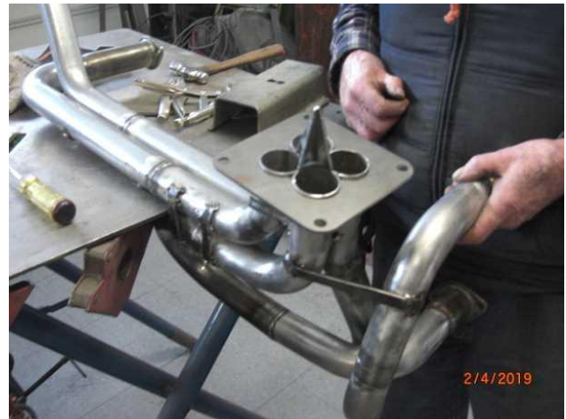
Fig. 9: Ron preparing to join the pipes with an interior flow separator that will go into the 4-into-1 collector.
