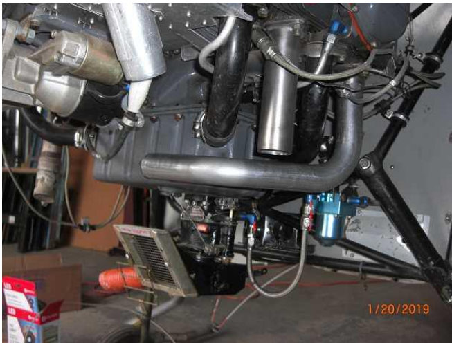
Fig. 3: Fitting the number 4 runner first – farthest from the collector location. The number 2 stack is in place as a guide for clearance.
