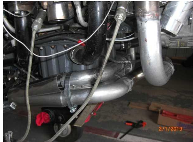
Fig. 6: The number 1 runner has been fitted into the collector and is waiting to be tack welded. Numbers 2 and 4 have been final welded. Note the braces between runners.
