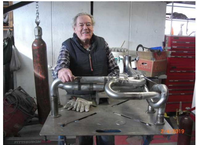
Fig. 10: Exhaust system nearing completion – what a handsome welder!
