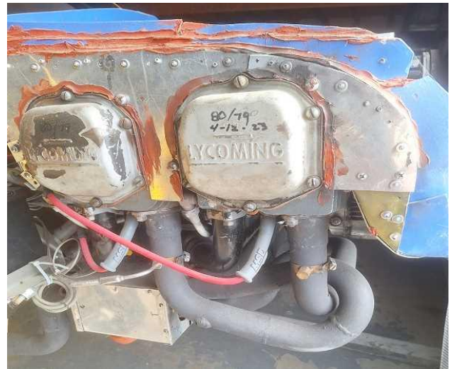
Fig. 13: Repurposed Tailwind exhaust system installed on Jodel. Note installation of Exhaust Gas Temperature (EGT) probe in the left pipe.
