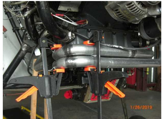
Fig. 5: The number 2 and 4 runners have been fitted into the collector and are clamped in place waiting to be tack welded.
