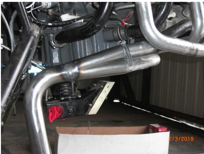
Fig. 8: Collector and exhaust pipe trial fitting. The exhaust pipe was subsequently cut up high to achieve a vertical angle.
