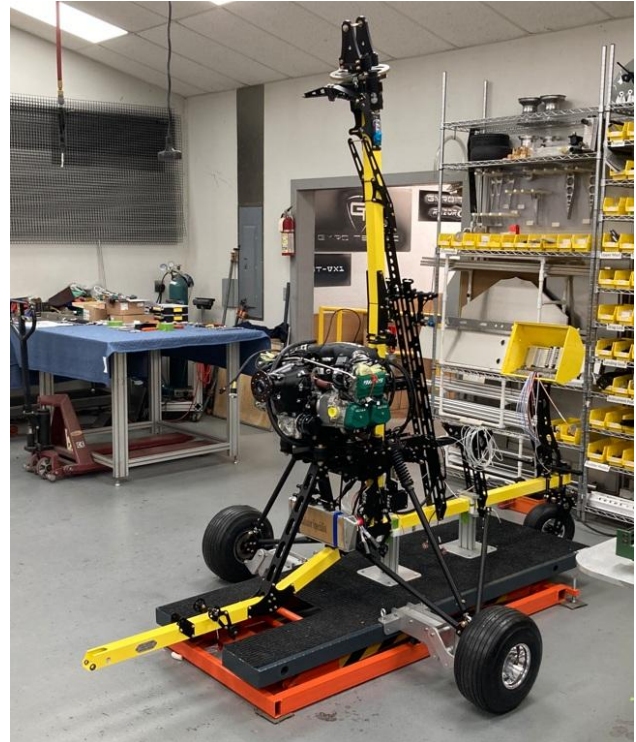
Partially completed airframe with Rotax 912iS mounted. I will share more assembly photos in the next issue.
