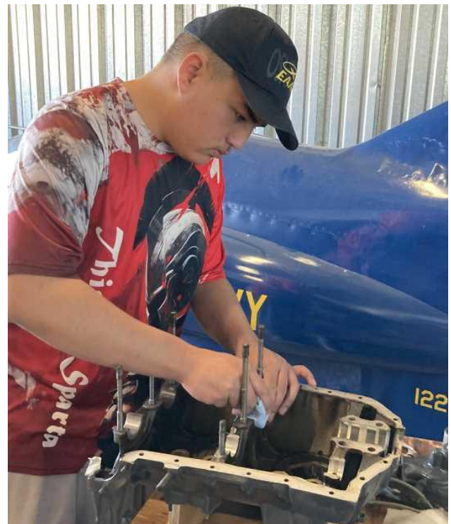
Logan assembles a Continental A65 engine under the guidance of Jim Nunnelee.
