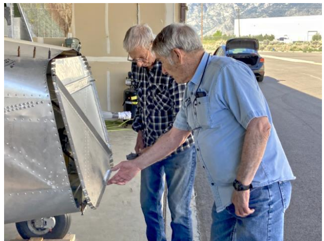
Jim and Cliff test-fitting the firewall to the fuselage.
